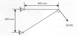
b) Develop the Finite Element Equation for the most general element using Rayleigh Ritz method for the mathematical model given
